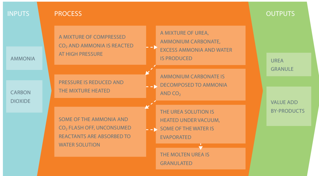
Figure 2.2 Urea fertiliser production overview
